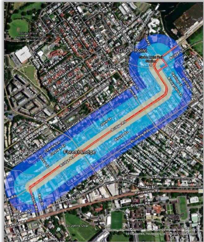
Figure 1: The Addendum REF reports on a construction noise assessment that modelled night-time construction noise for three residential zones – 'noise catchment areas' (NCA) around the construction area (p. 45). The colours represent the zones which are defined by distance from the construction. For the dark blue zone (NCA3 165 m), noise levels are expected to equal the acceptable level of 50 dB(A). For the light blue zone (NCA 2 105 m), at 55 dB(A), they're expected to exceed the acceptable 50 dB(A). For the closest zone (NCA 1, residences within 30 m of construction), the predicted noise level is 75 dB(A), which 'for residential receivers is considered 'highly intrusive' (p. 6).(See note 1)
