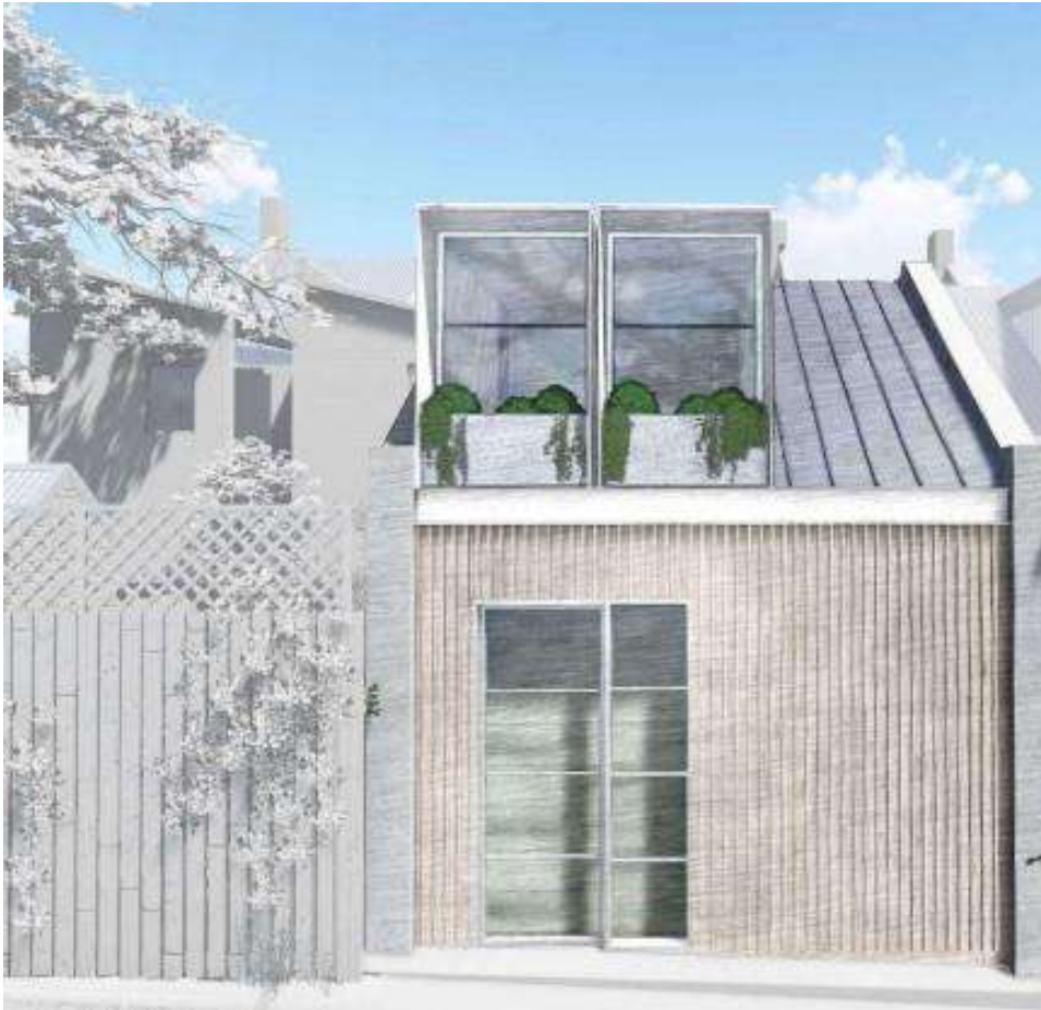
Figure 8 The Denman Lane elevation of the proposed building. The General provisions of the DCP state that A one storey structure with an attic above is permissible adjacent to a rear lane (Section 4.6.1 (1)). The proposed building is effectively not a one story structure but a two storey one and therefore does not comply.
