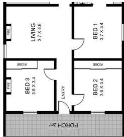
Figure 12 The plan of 181 St Johns Road is a standard mid-19th century cottage plan with the passage ending after the first range of rooms. It is very similar to the plan Joseph Elliott drew of his house in 1860 (see Figure 11). The room marked Bed 3 on this modern plan was most likely originally the parlour (plan courtesy realestate.com)
