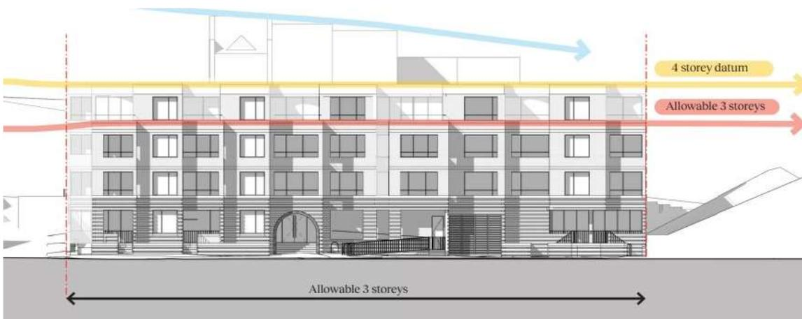
Figure 9 The proposed building exceeds the height controls in the LEP and the height in storey controls in the DCP.
