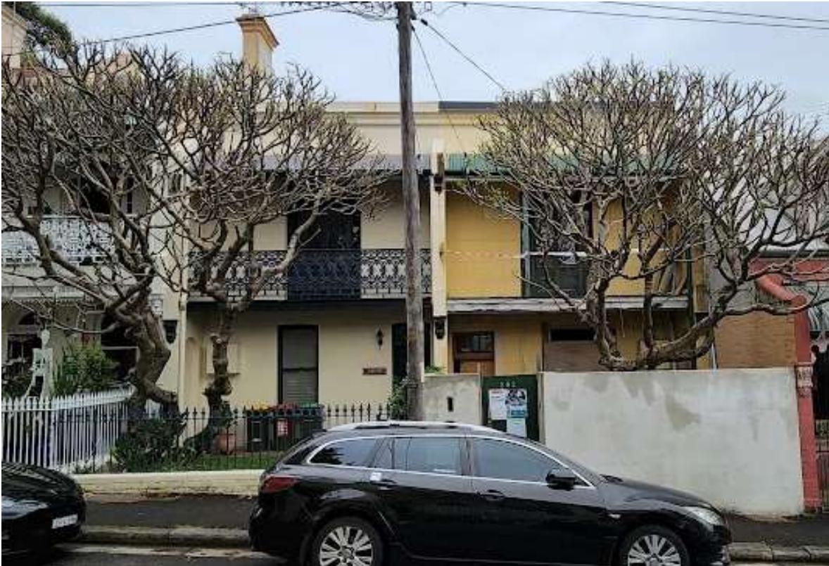
Figure 1 202 Hereford Street was built as a pair with 200 Heritage Street. 202 Hereford Street has a modern high brick wall on the street which should be replaced by a copy of the palisade fence of its neighbour
